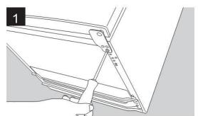
Undo the three screws in each bracket using the Phillips screwdriver.
